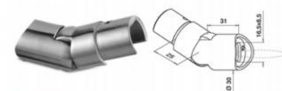
TU-06 Item NO \emptyset TU-06-424 42.4 for 24X24mm single slot
